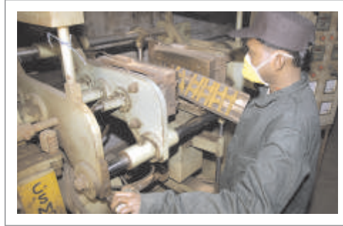
Shell Core Preparation
